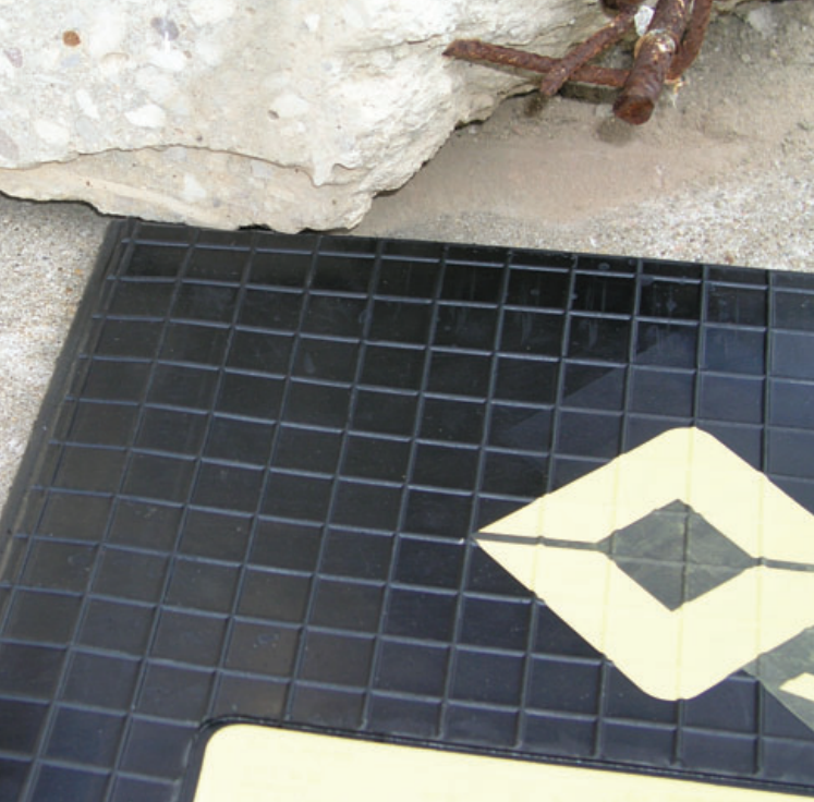
Mini-Lifting Bag, insertion height 2.5 cm. (1 inch)
